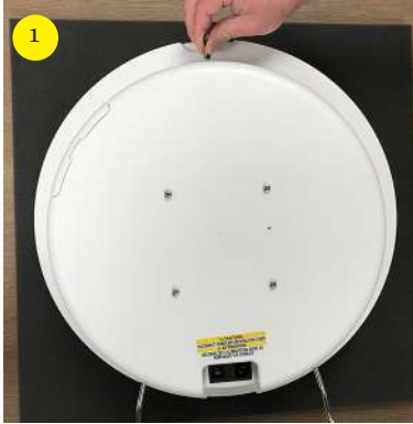
1 Remove top safety screw with the L-shaped TORX tool.
