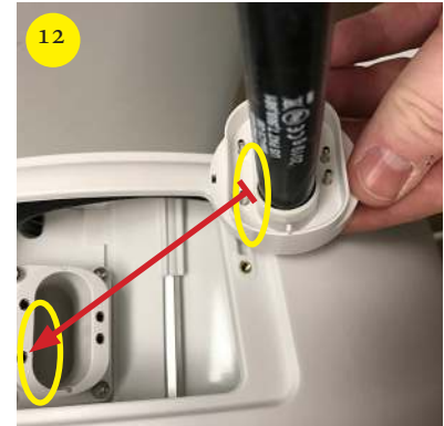
Match wide UV-A bulb pins to wide pattern in the bulb socket.
