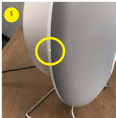
Green indicator will illuminate when the power is on.
