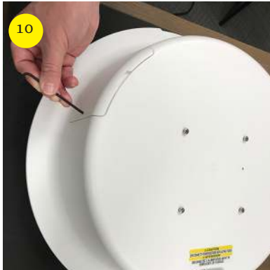
Remove UV bulb cover safety screw.
