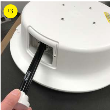
With wide pins on the left, insert UV-A bulb into bulb socket.
